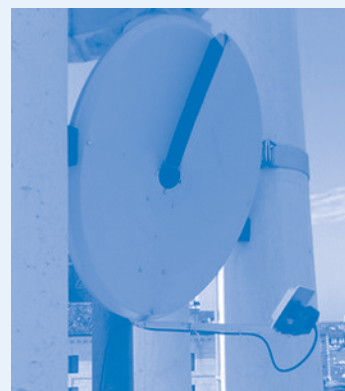
An orbital angular momentum (OAM) dish can spin vortex radio waves carrying parallel streams of massive data.
